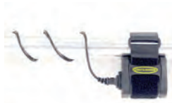
Figure 14: Cable coiled on frame.
